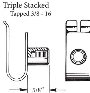
Cable Hangers are available in Mild Steel and Stainless Steel types 304 and 316.
