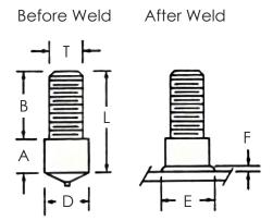
**Aluminum SB (Shoulder Base) welding studs** are partially threaded studs with a base diameter greater than the thread diameters. Available with weld-base diameters from 5/16" through 1/2'; thread diameters as specified.
