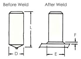
**Aluminum FB (Full Base) welding pins** are unthreaded fasteners. They are available in diameters from 1/4" through 1/2".
