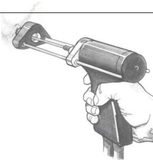
1. WELD PINS IN PLACE.
