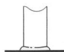
4. Metal solidifies & weld complete in milliseconds.
