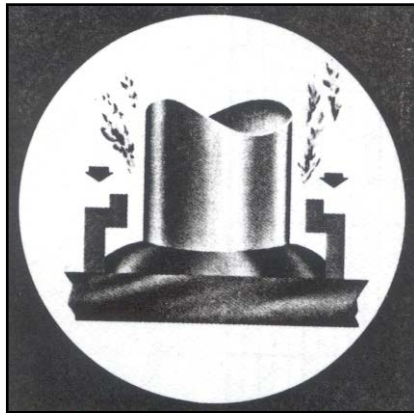
3. CONTROL TIMES OUT & STUD PLUNGES INTO MOLTEN STEEL.
