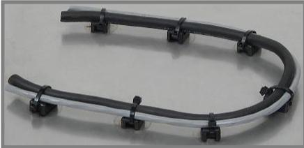
Wire Tie Down Studs were designed specifically for quick and rugged wire security and will hold wire bundles up to 1" in diameter. The Wire Tie Down Stud can be neatly welded into place within milliseconds providing a permanent, worry-free wire maintenance system.
